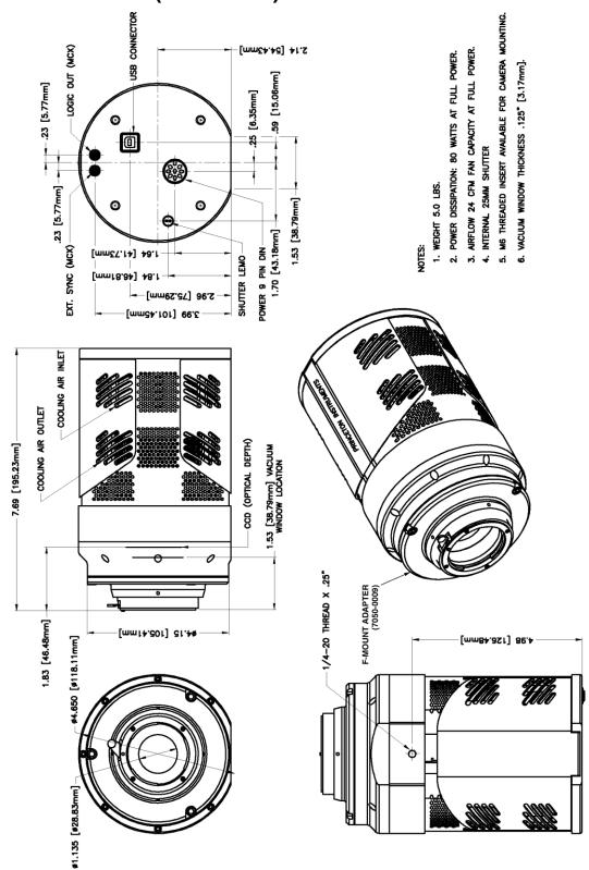
Figure 62. F-Mount: Internal Shutter (Air-cooled)
